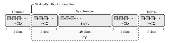
Figure 11: The stages of the protocol  $\pi_{\text{DPoS}}$  that use the blockchain as a broadcast channel in an epoch of  $R \ge 2k + 4\ell$  slots.
